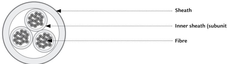
5.1.56. Examples of other typical fibre cross-sections are shown below.
